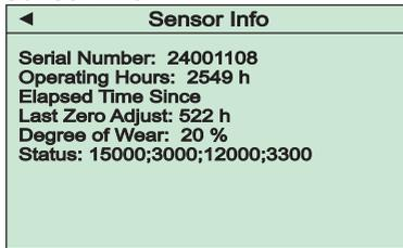
Under this menu item information regarding the sensor of your device is listed, for example parameters that will help to estimate the degree of wear and tear.
