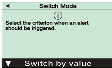
The thresholds to switch-on and switch-off the alert can be edited under menu “Switch Values”.
