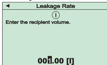
In the next step the internal volume of the vacuum vessel or system has to be entered. After confirmation of the adjusted value by means of the “OK” key the rate-of-rise measurement will be started continuously updating the calculated result for the leakage rate:
