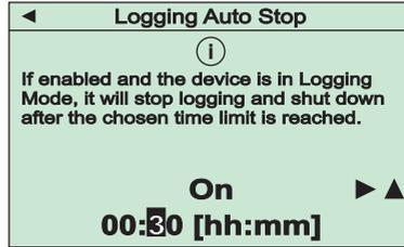
This function will terminate data logging automatically after an adjustable time limit.
