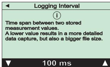
Measurement data will be stored with this adjustable time interval after the data logging is started. The edited value must finally be confirmed with the “OK“-key.
