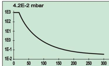
Depending on the diagram settings pressure readings will now be plotted over time. The current pressure reading is displayed numerically on top of the diagram.
