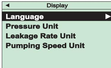
The menu is used to select menu language and display units. All settings must finally be confirmed with the "OK"-key.
