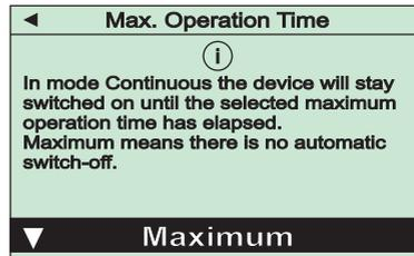
This function assures that the VD810 will be switched-off after an adjustable maximum operation time even in operation mode "Continuous". This will avoid unintended discharge of the battery. You can select "Maximum" (no switch-off) and pre-defined time periods between 30 min and 5 h.
