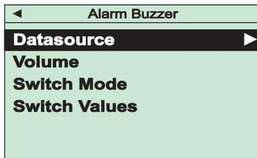
With this function an optic and acoustic alert function can be activated. Under “Datasource” you can initially activate the alarm buzzer and select which measurement signal should trigger the alert.
