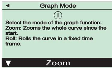
Under this menu item you can choose whether the pressure-over-time diagram will show all measurements beginning from the start of the plot ("Zoom") or whether measurements are plotted in a rolling mode within an adjustable time frame including the current reading ("Roll"). The setting must finally be confirmed with the "OK"-key.
