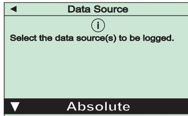
In this menu you can select the data sources for data logging, i.e. if absolute pressure, relative pressure or both should be recorded. The selection must finally be confirmed with the “OK“-key.
