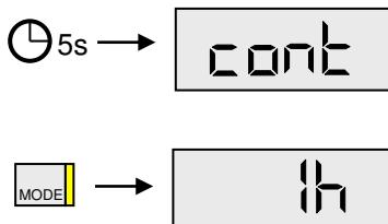
Using the Mode-Key you can now select a timespan from 1h to 24h or cont (no switch-off).
