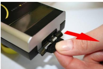
The sockets for the plug-in power supply and USB are located behind a protective rubber lid.
